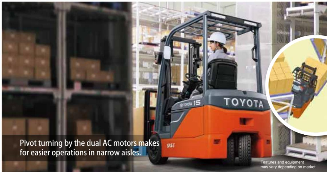
Pivot turning by the dual AC motors makes for easier operations in narrow aisles.
